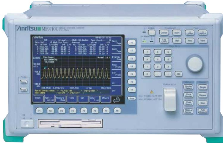
The MS9710C is a diffraction-grating spectrum analyzer for analyzing optical spectra in the 600 to 1750 nm wavelength band. In addition to uses such as measurement of LD and LED spectra, it has functions for measuring the transmission characteristics of passive elements such as optical isolators, as well as NF/Gain of optical fiber amplifier systems.
